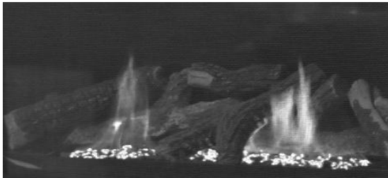
Proper Flame Appearance with logs
