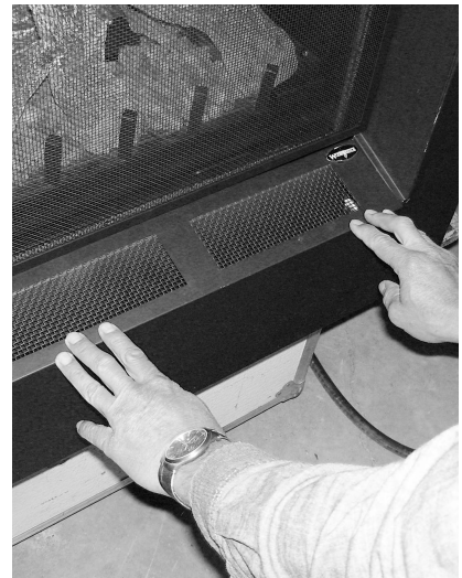
STEP 6: Tilt the Panel down to rest on the face support.
