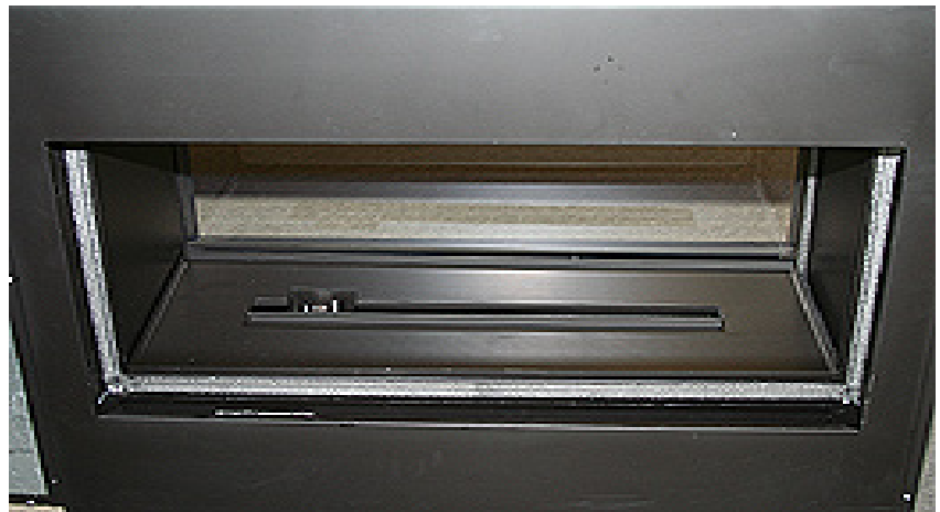
Figure 38 - Placing media tray
