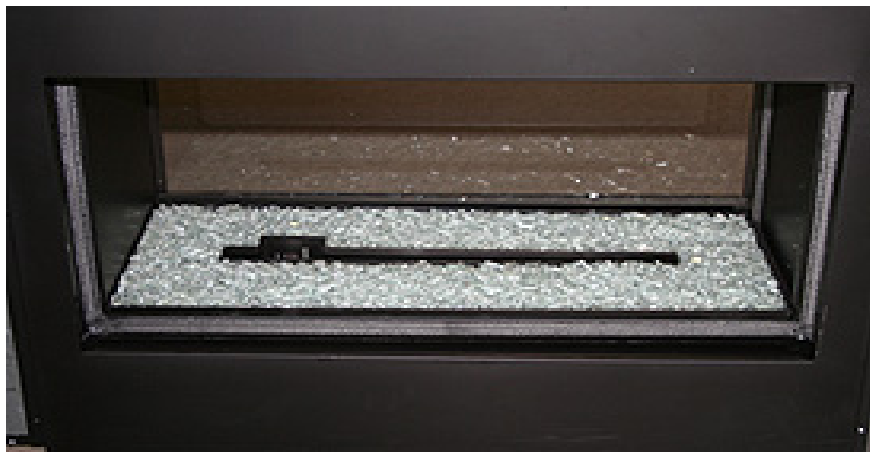
Figure 39 - Filling the tray with media
