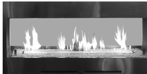
Figure 9 - Incorrect Burner Flame Pattern caused by port blockage
