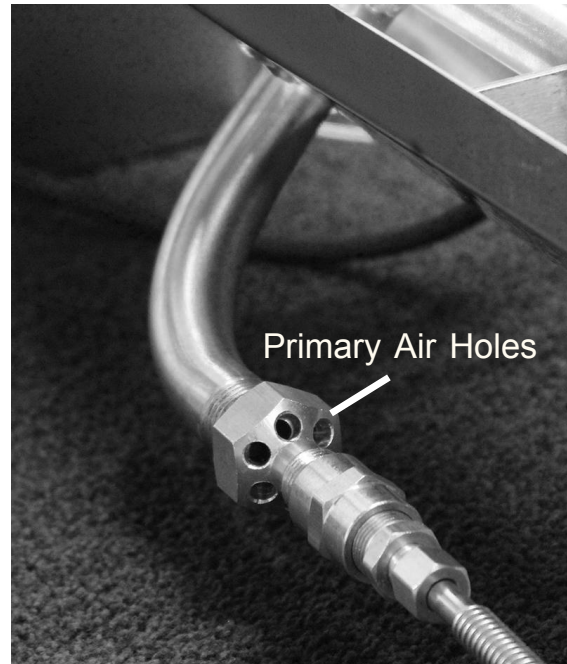
Figure 10 - Air Mixer/Injector on BurnerTube (propane models only)
